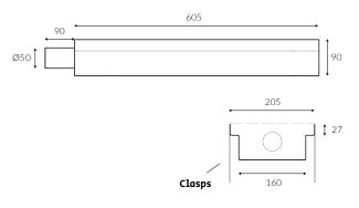
**600VLS** – with filter and sleeve for side connection and water trap.
