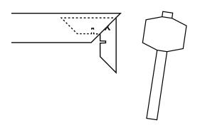
**3.** Place the A sides & fit the B sides by sliding both corners together. Use a rubber mallet or hammer with a wooden block (which acts as spacer).
