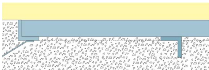
Casting frame with strut to avoid getting hourglass shape of the frame.
