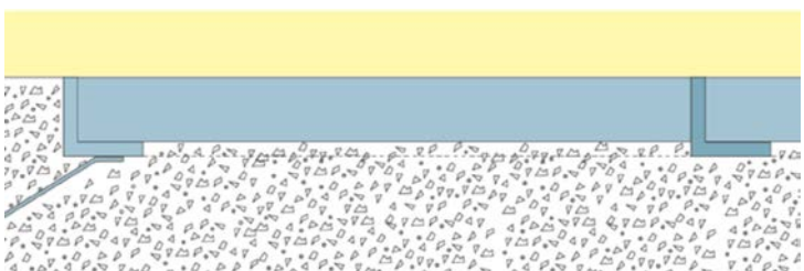
Casting frame with dividing strut.
